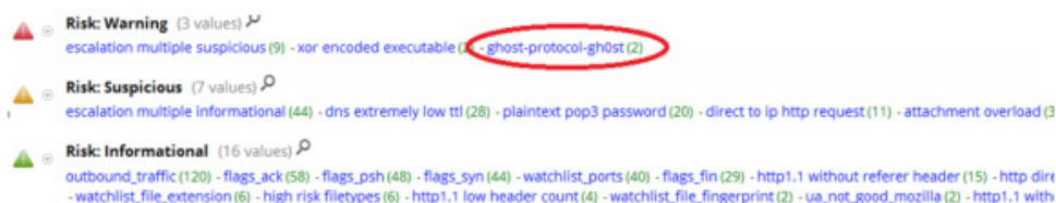
Figure 1 – RSA NetWitness logs and packets detects Gh0st protocol network traffic
