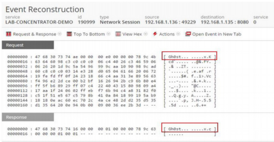
Figure 2 – Reconstruction of Ghost payload in RSA NetWitness logs and packet
